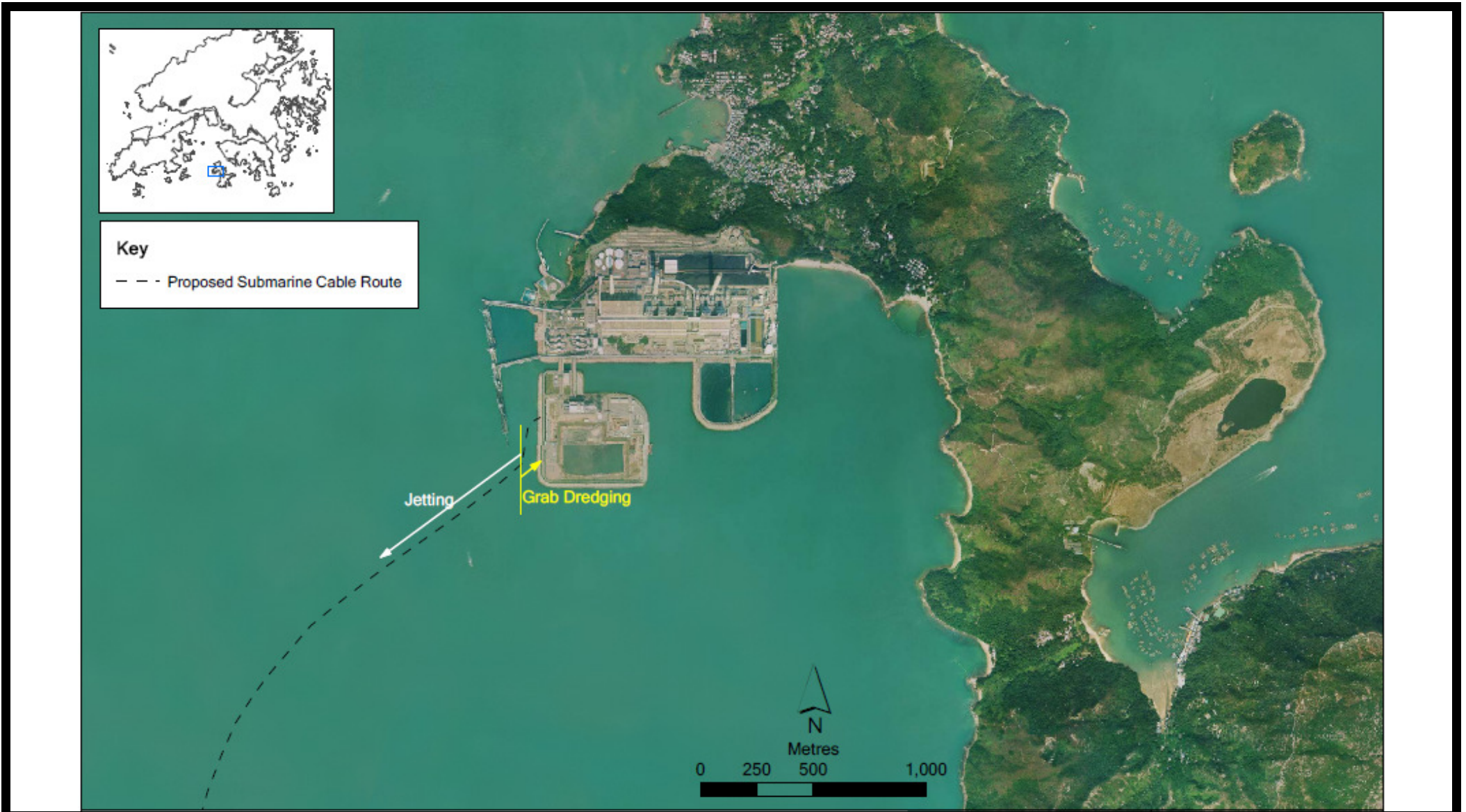
Figure 2: Zones of Dredging and Jetting (Prepared based on Figure 5.9 of the EIA Report)
